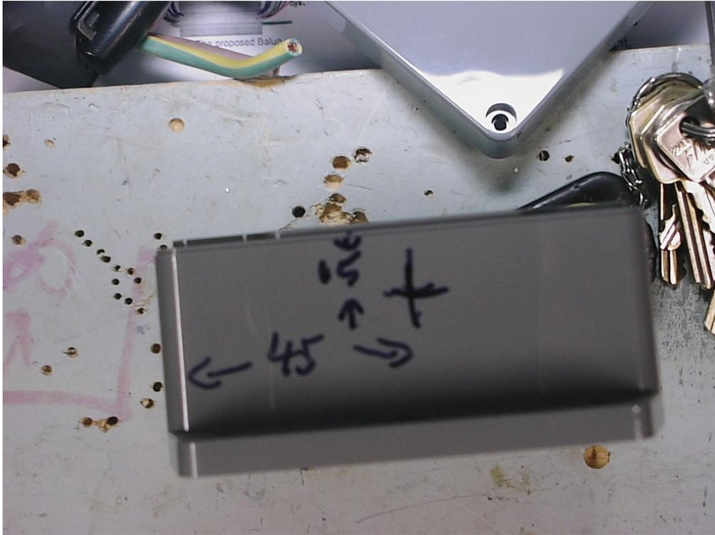
Drill a hole to suit your selected socket type. I used a small hole saw to suit the SO239 panel mount socket
