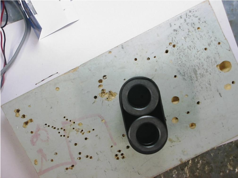
A paint stripper heat gun (on low) shrinks the tube quite well.
